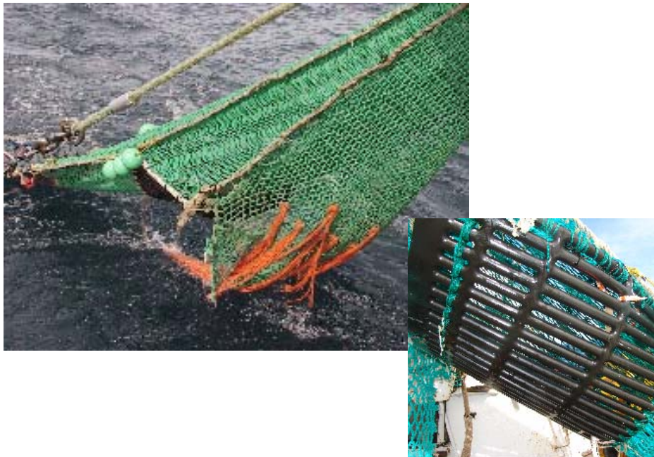
Figure 3.: Photos of the selective trawl fitted with a 20mm bar spacing grid
